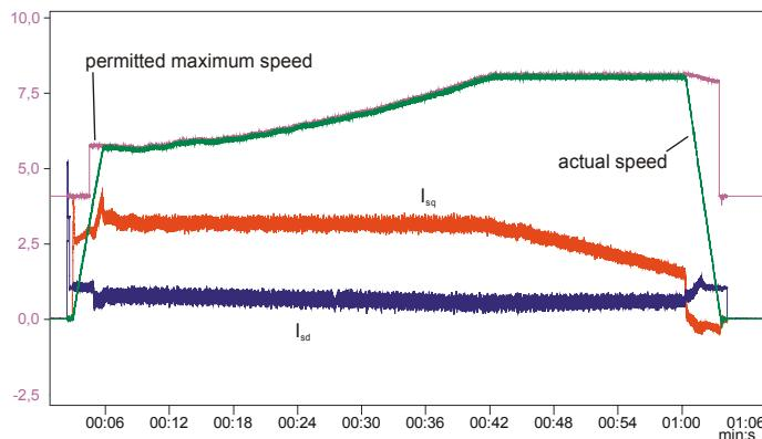
The rise of the torque-forming current  $I_{sq}$  at the 6 s point in time is needed for the acceleration.
