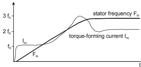
If the parameter *Operation mode LE 822* is set to 3 or 4, the additional current for the acceleration is taken into account. In this, the limit current is the effective value of the stator current which can be set for a short time during the set maximum acceleration. As the deceleration is regarded as being particularly critical, the set *Deceleration Anti-clockwise 423* is taken into account here.
