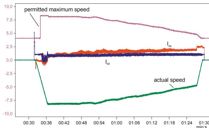
The permitted maximum speed is displayed in the above illustration with the negative speed in an anti-clockwise direction.
