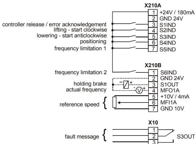
**Note:** The connection diagram describes the standard configuration of the control terminals. According to the requirements in the application deviating connection possibilities are to be configured by the freely programmable combinations.
