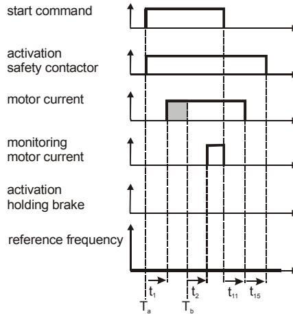
If a new start command is given before the sequence for stopping has ended, the last step of the sequence is canceled immediately. The described start sequence then commences, starting with this condition.
