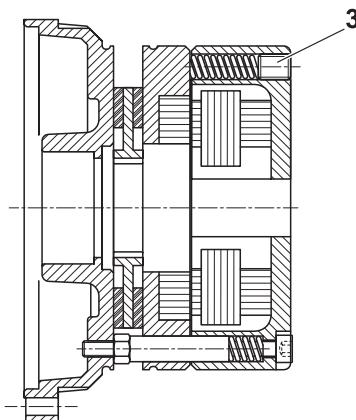
Brake torque can be adjusted steplessly by changing the preload of springs (3).
