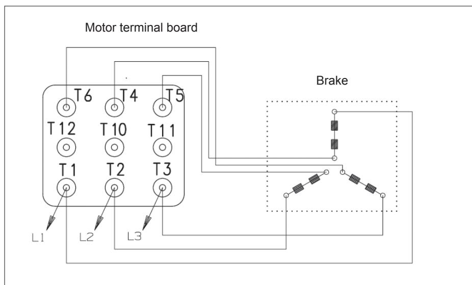
Switch-pole motors, nine pin motors (BX, BE, BN, MX, ME, M, MNN) and, at request, single-pole motors with separate power supply are equipped with an auxiliary terminal board with six terminals for brake connection.
